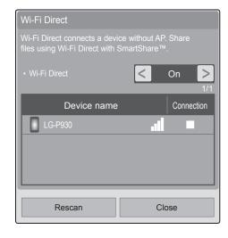
Wi-Fi Direct pop-up window display is the same whether the TV is or is not in Pass-through Mode.
